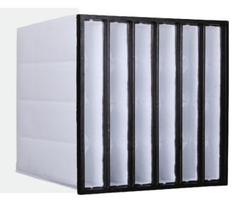
Material – Multilayers of 100% Polyester PET Synthetic fibers – Self supported Pockets Construction – Thermally Bonded Rigid pocket Media have Aerodynamic internal diamond spacers for Aerodynamic flow, to ensure the proper Airflow distribution.
