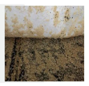
Media Constituents - Activated carbon and Ion exchange resin or blend of both bonded to non-woven synthetic substrate.
