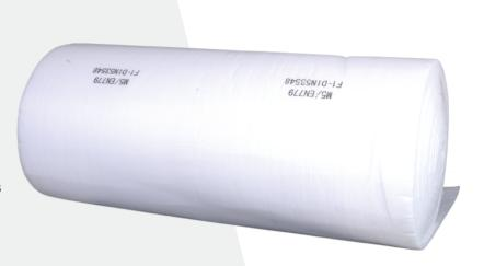
Material - 100% PET PP Nonwoven Synthetic Fibres , Needle Punched, Thermally Bonded Construction - By arranging progressively structured Media fibres with Fully tackifier and PP/Glass Scrims Grades - M5 & M6 / MERV 10 & MERV 11 / ISO ePM10 to ISO ePM 2.5
